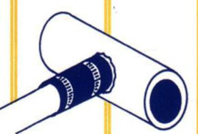
Tighten screws to 60 in./lbs. torque
