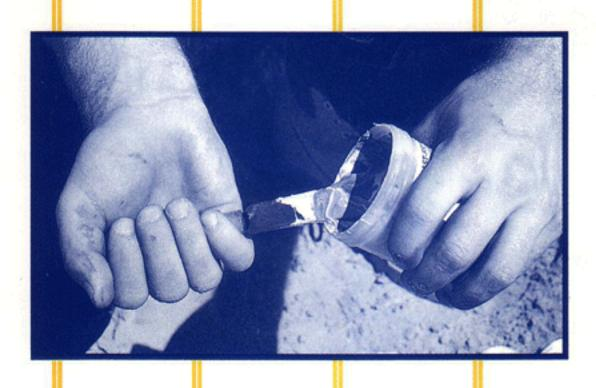
The epoxy kit, supplied with each Fast-Fit Tap Saddle, sets up in minutes and may be used in wet or dry conditions. Simply mix together thoroughly.
