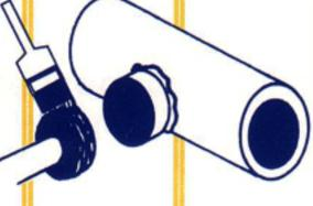
Insert donut & spigot assembly into opening & drive with hammer
