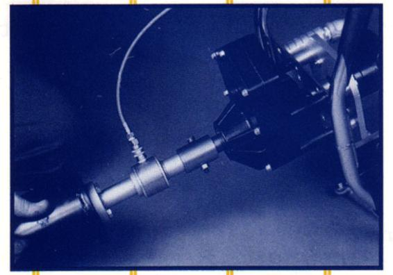
Connect Shell Cutter, arbor and water supply to power unit.
