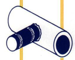
Insert pipe into coupling
